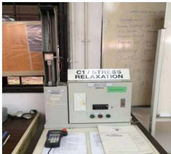
Figure 1. C_1 /Stress relaxation machine
