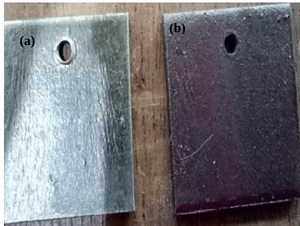
Figure 1. (a) Low carbon steel coupons and (b) Stainless steel 304 coupons
