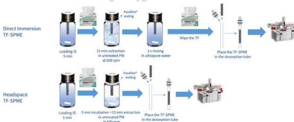
Figure 3. Scheme of the tf-SPME configuration [51]
