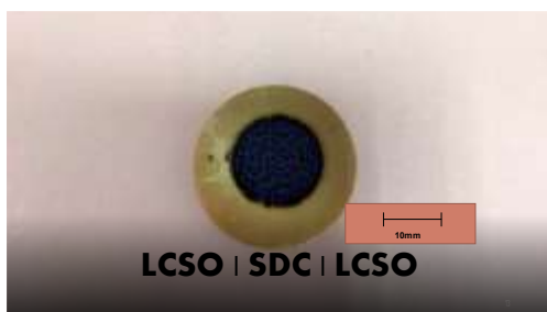
Figure 3. Prepared symmetrical cell LCSO|SDC|LCSO
